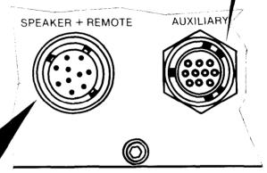
Provides connection for an audio input to the modem and for an audio output to loudspeaker. May be used with other equipment for remote operation.
