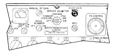
Check meter for direct current (20 or 60 mA) flowing through DC LOOP NO. 1
