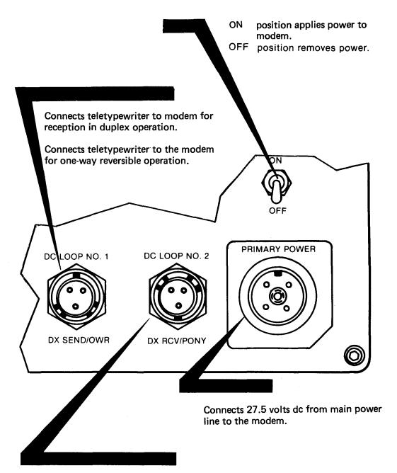
Connects teletypewriter to modem for reception in duplex operation.
