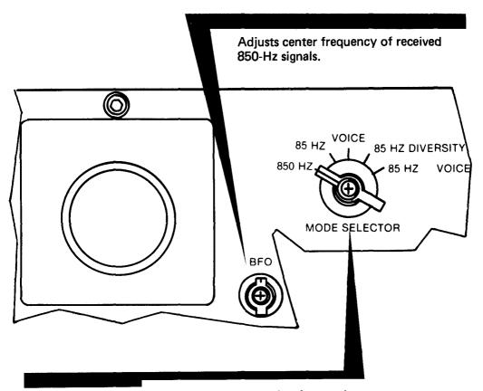
The position of this switch selects the mode of operation.
