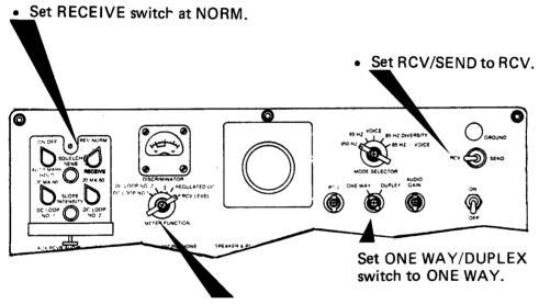
Set METER FUNCTION at RCV LEVEL.
