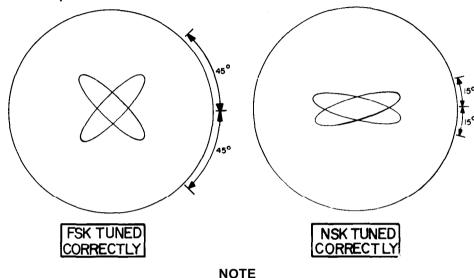
When the modem is warmed up, 5 minutes will be necessary for the BFO to stabilize. If the modem is cold, 15 minutes will be necessary for BFO to become stable. Make necessary adjustments during these time periods to maintain the best signal reception display on the scope.
