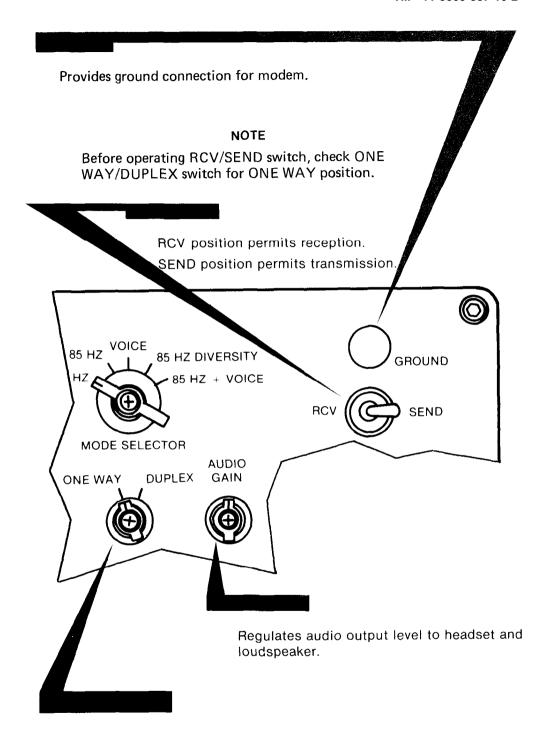
ONE WAY position permits either reception or transmission. DUPLEX position permits reception and transmission at the same time.
