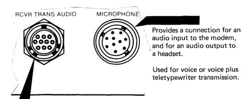
Used in duplex and one-way reversible operation to connect audio output circuit from modem to exciter section of receiver-transmitter.
