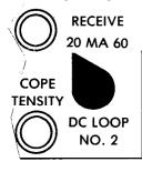
Set DC LOOP NO. 2 switch at 20 or 60 MA, as needed.
