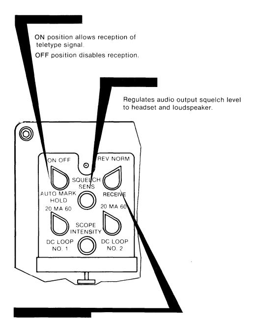
NORM position allows reception of teletype signal by use of normal mark-space polarities.
