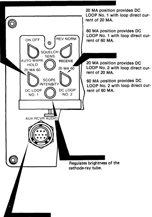
Used in duplex operation to connect audio output of auxiliary receiver to modem.
